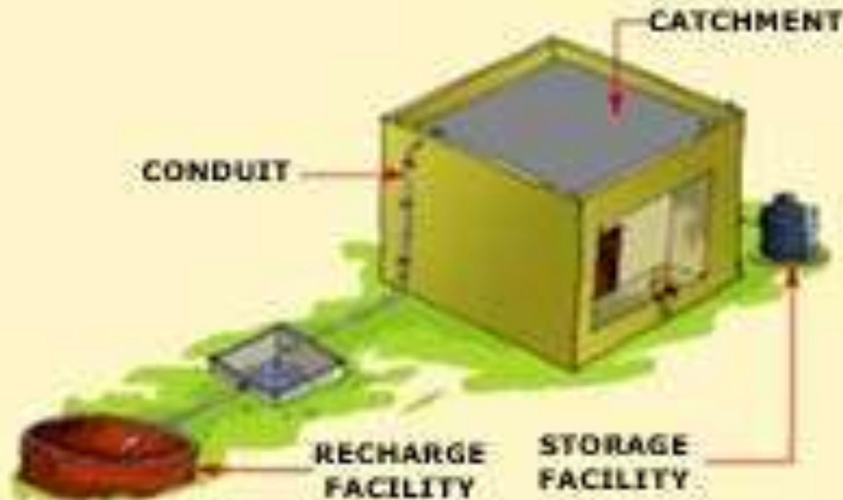
ELEMENTS OF A TYPICAL WATER HARVESTING SYSTEM
